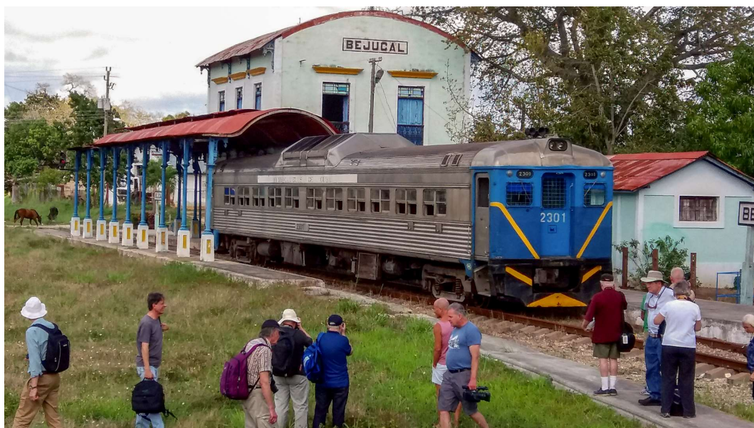
The Budd Rail Diesel Car (RDC) is a self-propelled diesel multiple unit (DMU) railcar
