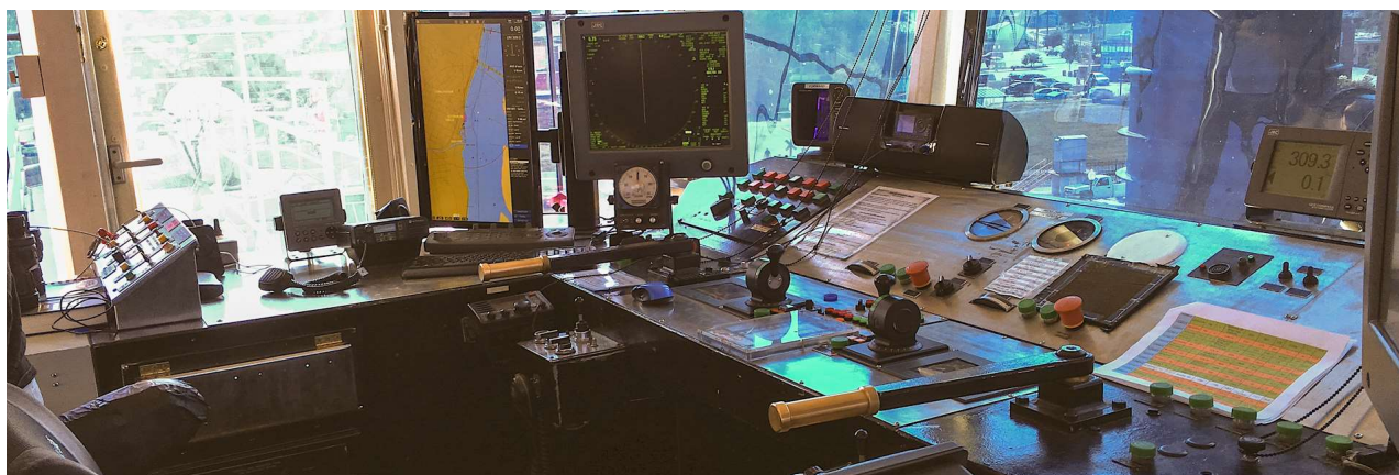
The pilot house also known as the green bridge on the American Queen
