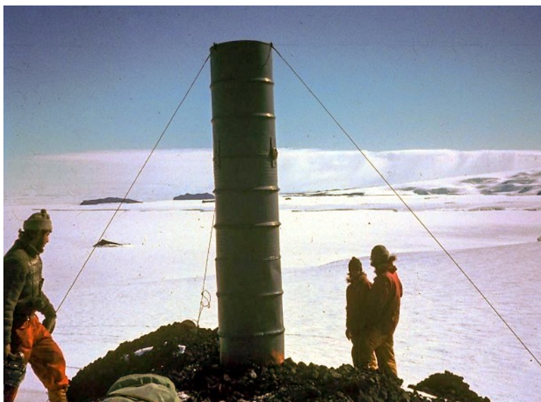
Survey beacon made from 44 gallon drums
