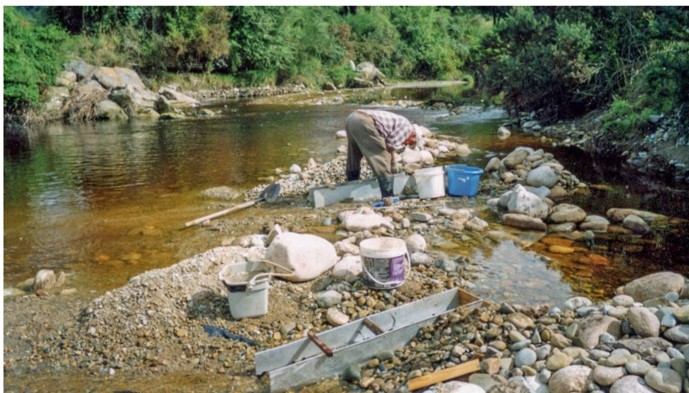
Neil fossicking for gold in a stream with his shovel, two buckets and home made sluice box. Neil is standing over his sluice box. One of Neil's mates is using the other sluice box and buckets.
