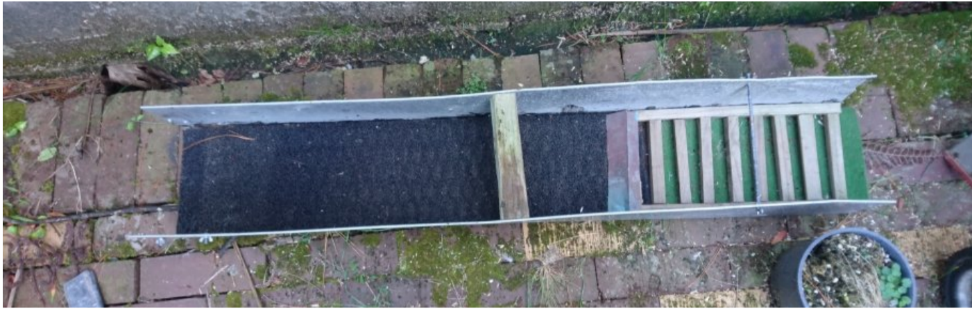
Neil's original sluice box. The material being sluiced is put onto the black miner's moss mat. Water flows in over the black miner's moss and then down over the riffles. Gold is trapped in the black matt and in the green material under the riffles.
