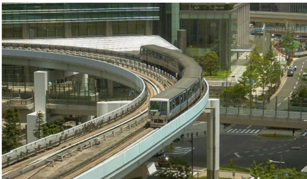
The Yurikamome train is controlled entirely by computers with no drivers on board.
