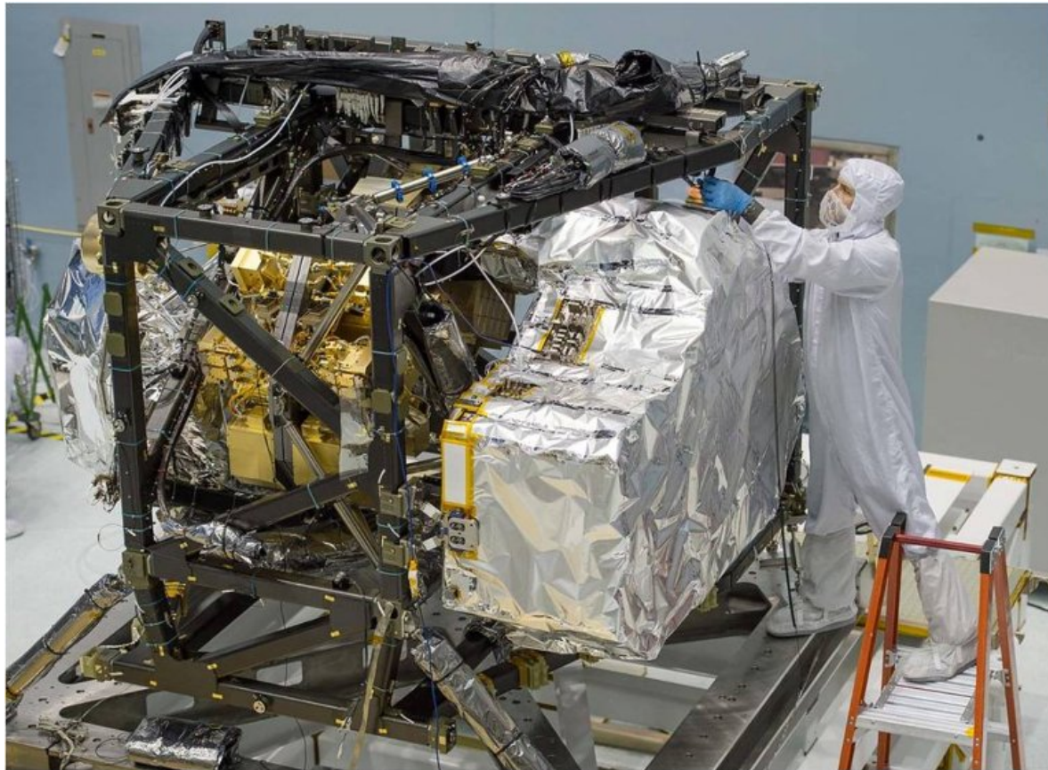
Four scientific instruments are packed together in the instrument frame behind the primary mirror
