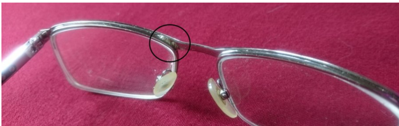
Titanium weld on the inside of my metal glasses frame done by SOS Eyewear
